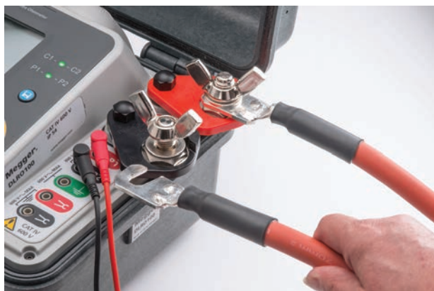
A terminal adapter has been designed to enable the use of user's own test leads.
