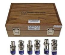
Maury precision BNC VNA calibration kits include each of the calibration standards and tools shown in the tables at the right. Between-series adapters are sold separately.
