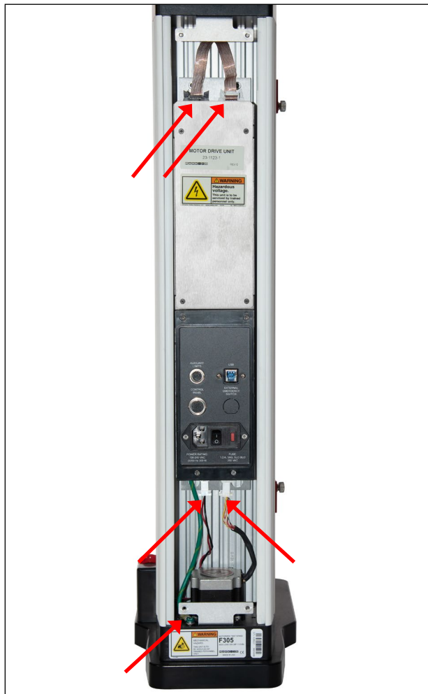
Locations of connectors, ground wire, and bracket
