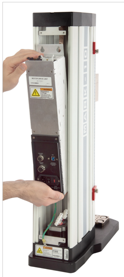
Removing the electronics module
