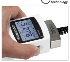
^ The Plug & Test<sup>®</sup> connector locks into the receptacle in the indicator when fully inserted. Dual buttons on the indicator housing release the connector for easy removal. Gold plated spring contacts ensure long lasting and reliable connection.
