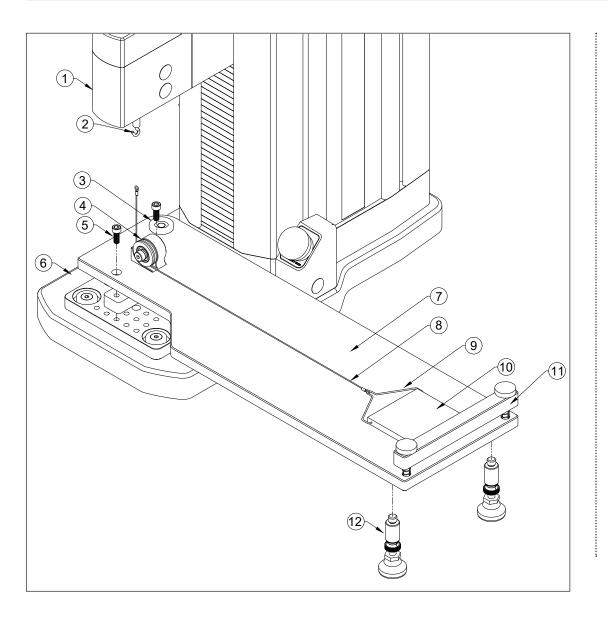
The G1086 COF fixture is designed for use with the following test frame models: F105, F305, F505, F755, F755S, ESM303. Adapters available for other models. The G1086 can be used for a wide range of materials, and conforms to ASTM D1894 and relevant standards. The illustration at left depicts proper assembly. Please follow these instructions:
