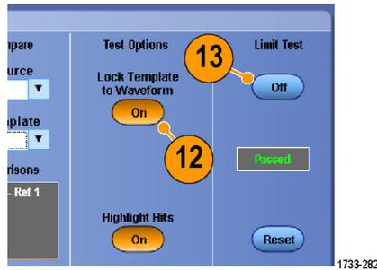
The instrument compares every waveform it acquires against the template until a waveform fails to match the template. When a failure occurs, acquisitions stop and the violations appear in a different color on the display. The following example shows Ch 1 on top so that you can see Ch 1, the template, and the hits.
