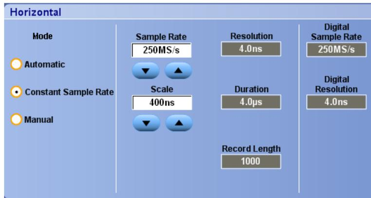
In Manual mode you can set the Sample Rate and Record Length. Horizontal Scale is a dependent variable calculated from the sample rate and record length. Masks are not supported in manual mode.
