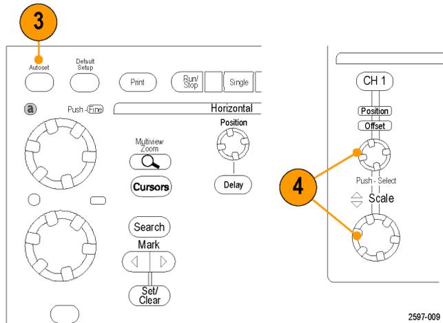
5. Adjust the horizontal position and scale using the front-panel knobs. The horizontal position determines the number of pretrigger and posttrigger samples.
