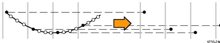
**Peak Detect** mode uses the highest and lowest of all the samples contained in two consecutive acquisition intervals. This mode only works with real-time, noninterpolated sampling and is useful for catching high frequency glitches.
