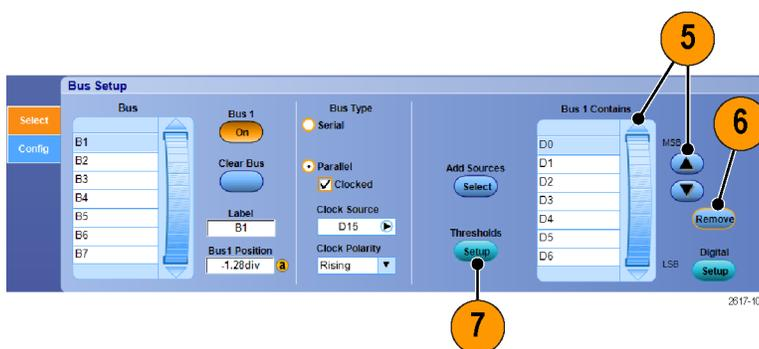
8. For each threshold you want to set, double click the channel Threshold, and enter the threshold using the keypad or multipurpose knobs.
