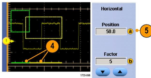
6. To adjust the zoomed area vertically, select **Vertical > Zoom Setup...**, click a vertical field, and then use the multipurpose knobs to adjust the Vertical Position and Factor.
