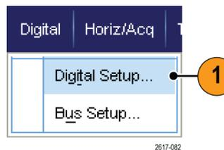
2. Select the **D7 - D0** or **D15 - D8** tab for the digital channels you want to set up.
