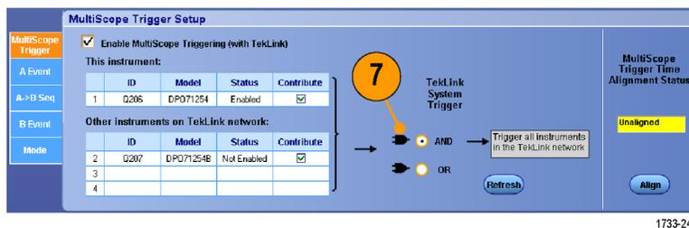
8. To align the MultiScope Trigger, press the **Align** button.
