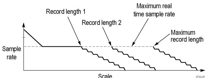
Automatic and Constant Sample Rate modes are identical. However, Constant Sample Rate mode keeps the sample rate constant at a rate that guarantees bandwidth enhancement filters are used.
