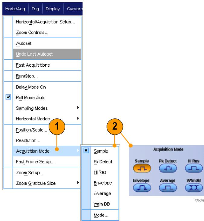
3. For Average or Envelope acquisition modes, click the **# of Wfms** control, and then set the number of waveforms with the multipurpose knob. For WfmDB mode, click the **Samples** control, and then set the number of samples with the multipurpose knob.
