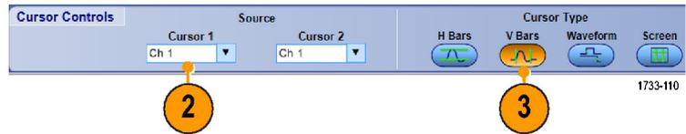
4. To take measurements between two waveforms, select **Waveform**, and then select the waveform source for each cursor.
