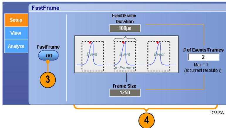
5. Use the Frame Viewing controls to select the frame that you want to view.
