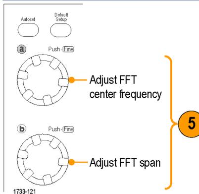
6. You can view time-domain and frequency-domain waveforms simultaneously.
