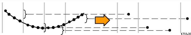
**Envelope** mode finds the highest and lowest record points over many acquisitions. Envelope uses Peak Detect for each individual acquisition.
