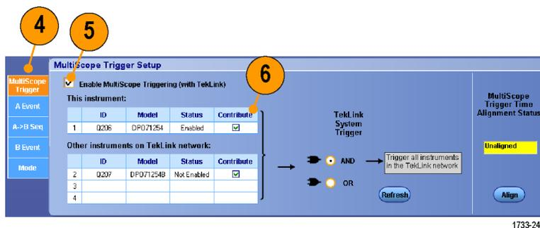
7. Select **AND** or select **OR** to combine all contributed triggers before triggering all instruments in the TekLink setup.
