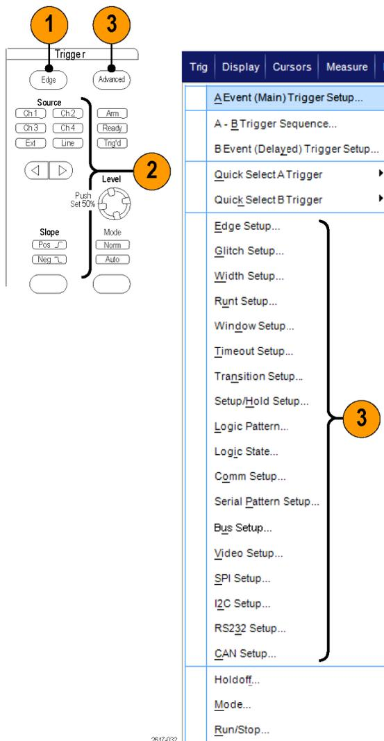
4. Complete the trigger setup using the controls displayed for the trigger type. The controls to set up the trigger vary depending on the trigger type, instrument model, and options.
