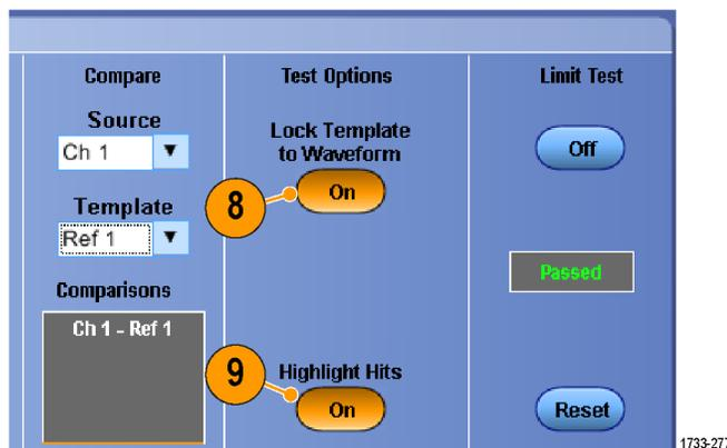
10. Toggle Limit Test to **On** to start the test.
