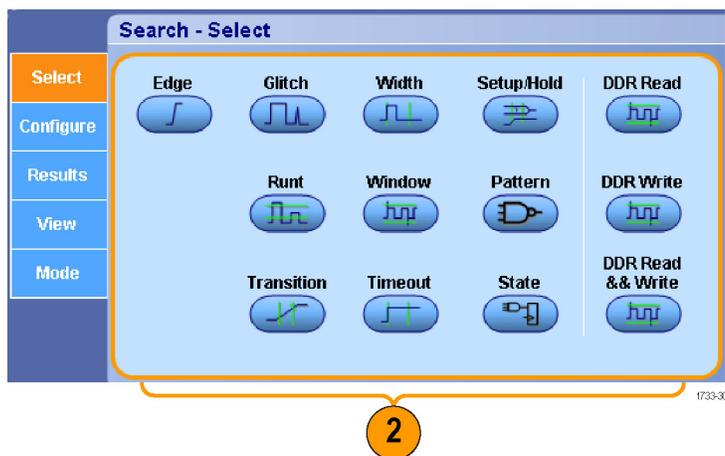
3. Set up your search from the Configure tab. To copy the trigger setup or a search setup, press Settings Copy.
