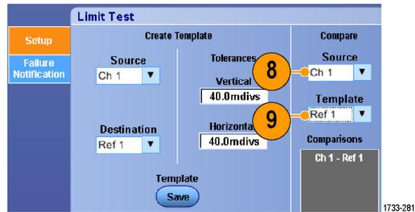
10. Click **Failure Notification** to set up the Failure Notification.
