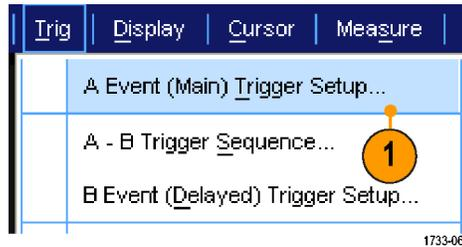
2. Set the A trigger type and source in the A Event tab.
