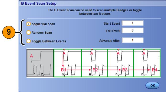
10. In this example, a DDR3 DQS signal is on Ch 1 and the DQ signal is on Ch 2. The instrument is in Run Mode with Display Mode set to Infinite Persistence. The instrument trigger setup was as follows:
