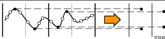
**Hi Res** mode calculates the average of all the samples for each acquisition interval. Hi-Res provides a higher-resolution, lower-bandwidth waveform.
