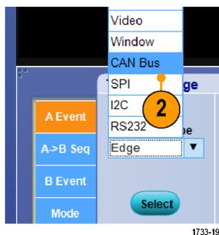
3. Select **Trigger On** to select the desired trigger on feature.
