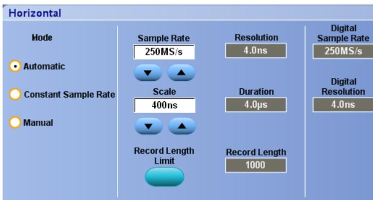
To set the Record Length Limit, click **Record Length Limit** and set the limit using the buttons or keypad. The default maximum limit depends on your instrument model and record length option.
