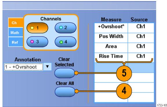
You can also choose a measurement for the selected waveform directly in the Measure menu. (See page 99, *Automated Measurement Selections*.)
