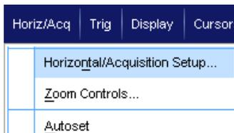
In Automatic mode you can set the Scale and Sample Rate. Record length is a dependent variable. If changing the scale would cause the record length to exceed the Record Length Limit, the sample rate is decreased to the next available setting.
