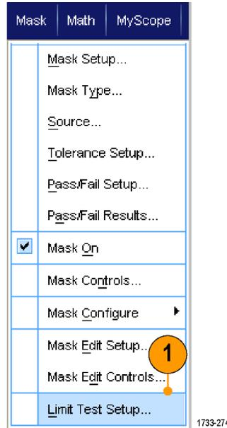
2. Create the template by selecting the Source, Destination, and Tolerances. Use the multipurpose knobs to adjust the Tolerances. Tolerances specify how much margin the signal is allowed before failing the limit test.
