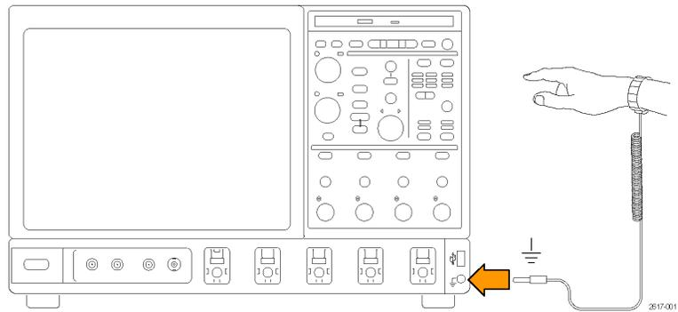
2. A cable that is left unconnected on a bench can develop a large static charge. Discharge the static voltage from all cables before connecting them to the instrument or device under test by momentarily grounding the center conductor of the cable, or by connecting a 50 Ω termination to one end, prior to attaching the cable to the instrument.
