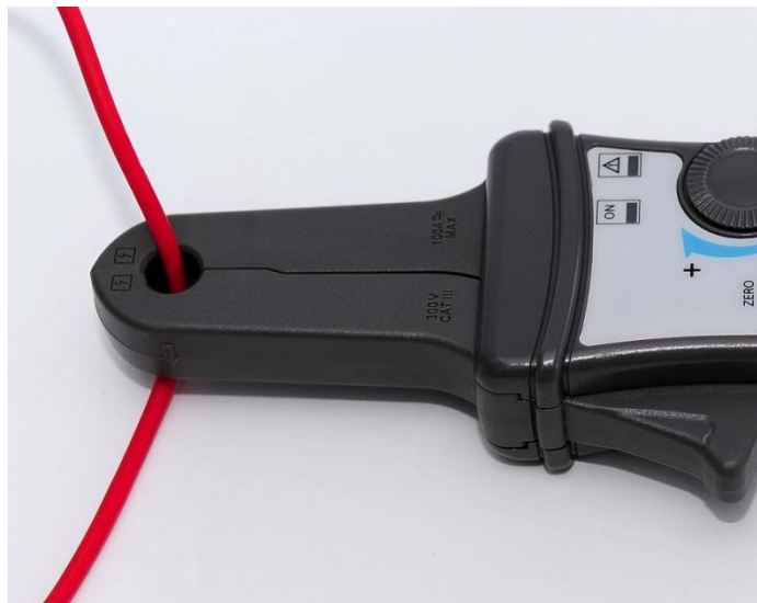
Figure 5: Connecting the CP62 current probe.
