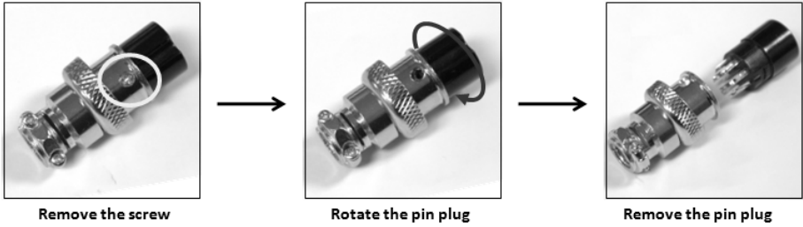
Figure 4 - Remote Control Connector
