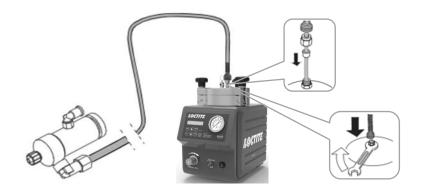
If two dispense valves are used, remove blanking plug from the reservoir lid and replace with additional reservoir/tube fitting.
