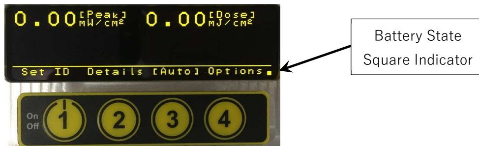
Image 13: Battery Status, Square Indicator
