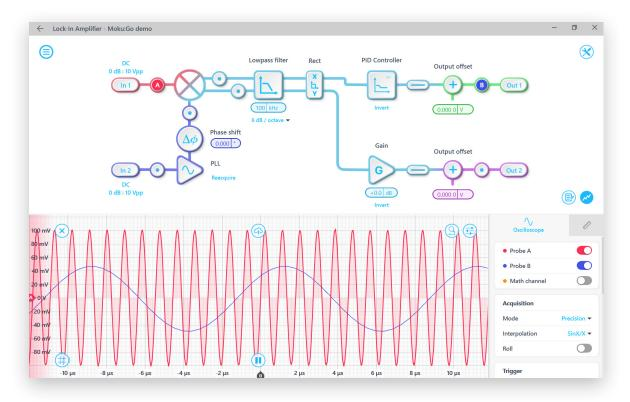
Demod. Frequency 1 mHz to 20 MHz Time Constant 128 ns to 2.15 s Filter Slopes 6, 12, 18, 24 dB/Oct
