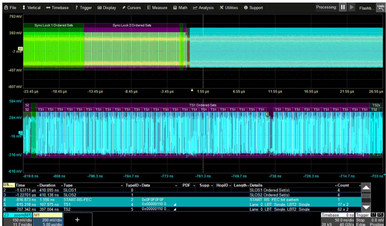
USB4 decoding shows the SLOS preceding the START-RS-FEC and the TS1 ordered set.
