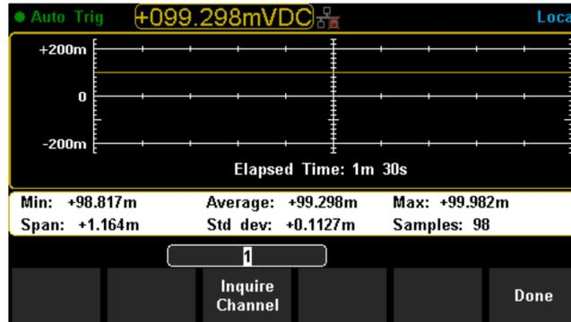
Set the [Inquire Channel] by direction keys and the interface displays the minimum, average, maximum, span, standard deviation, samples and trend chart of measurement results of the setting channel during the scan operation. Press [Done] to return to higher level menu.
