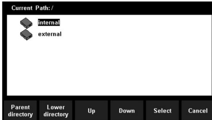
Use direction keys or menu operation keys to choose the state file with the suffix “.xml”.
