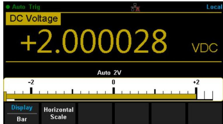
2. Press [Horizontal Scale] to set the vertical scale as Default Manual mode.
