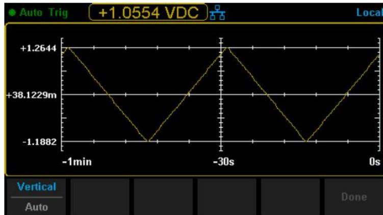
Press [Manual] and you can set the vertical scale manually, as displayed in the diagram below.
