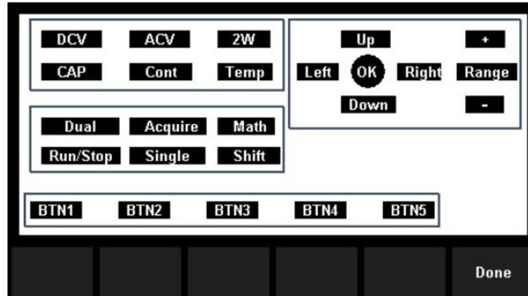
Before testing the keys the key shapes on the screen will be displayed in a blue color. The on screen keys and knobs will change to a green color when tested. Press [Done] to exit the test.
