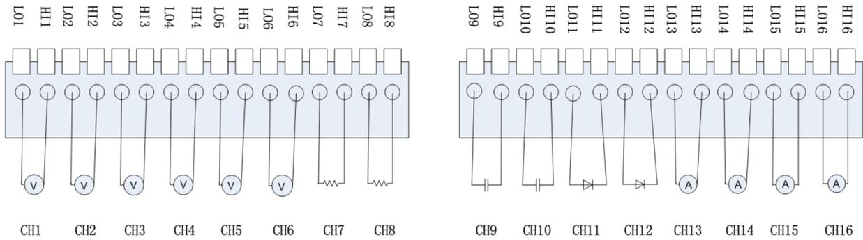
First 12 channels can be used to measure DCV/DCI ACV/ACI/CAP/FREQ/DIODE/CONT/TEMP and the last 4 channels are dedicated to current measurement.
