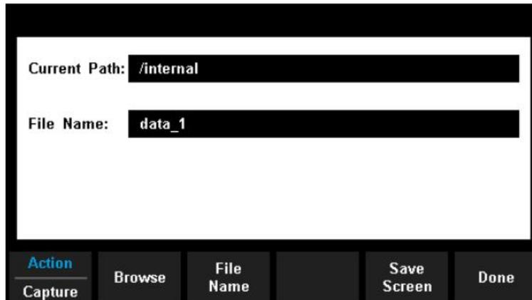
Press [Action] and select [Folder], [Capture Display], [Copy], [Rename] or [Delete] to do the corresponding operation.
