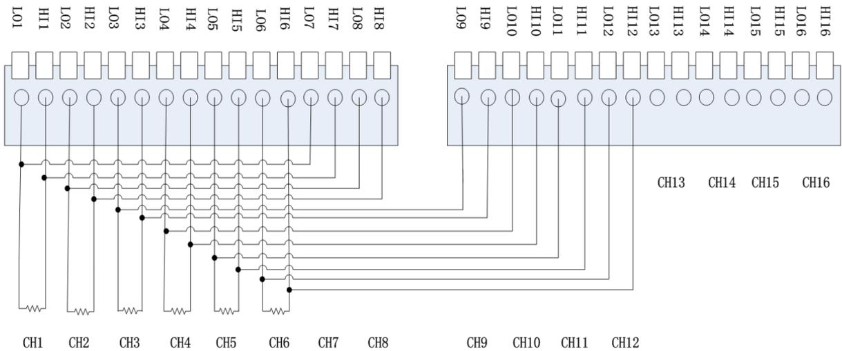
CH1 to CH6 can be used for measurements and CH7 to CH12 can be used as sense channels. To minimize voltage errors, the remote sense connections (CH7,CH8 etc..) should be made as close to the device-under-test (DUT) as possible.
