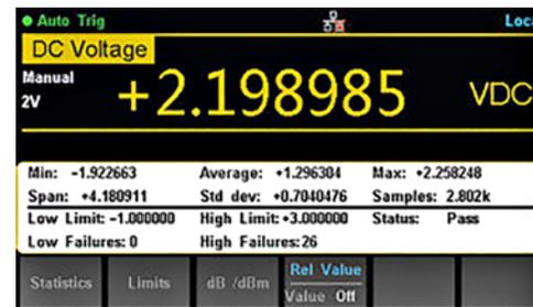
Statistics mode quantifies the data being captured while the Pass/Fail mode can quickly test, and instantly indicate if there is a problem.
