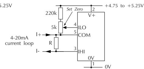
Measuring a 4-20mA loop current.
