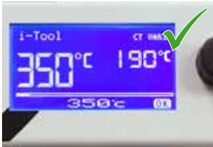
340 – 360 °C for lead-free solder
