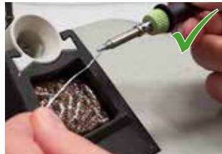
Add new solder after cleaning
