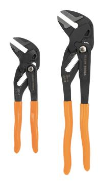
The 2-Piece Compact Plier Wrench Set includes 7-Inch (Cat. No. D5317) and 10-Inch (Cat. No. D53110) Compact Plier Wrenches with parallel jaws for a secure, damage-free grip on nuts, bolts, and workpieces. A quick-adjust button enables easy, one-handed jaw adjustment, while the high leverage ratio ensures strong grip and bending power. Laser-etched size markings make finding the right jaw opening simple and convenient.
