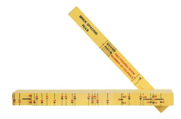
Klein Tools' 6-Foot Brick Fiberglass Folding Ruler is constructed of tough nylon, reinforced with glass fibers for added durability, and resistance to weather, abrasion, and most chemicals. Inch measurements are marked on both edges of the outside faces of the rulers, graduated to 1/16-Inch (1.6 mm). Standard brick scale measurements are marked on the inside faces of the rulers. Graduations are engraved on both sides with brick scale units on the other side for versatility.
