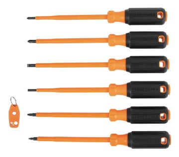
This 7-Piece Insulated Screwdriver Set, Made in the USA, includes assorted Klein Tools Phillips (Cat. Nos. 6856INS, 6836INS), slotted (Cat. Nos. 6816INS, 6826INS), and square (Cat. Nos. 6886INS, 6846INS) tip screwdrivers, plus a magnetizer (Cat. No. MAG2). Each screwdriver is individually tested to exceed IEC 60900 and ASTM F1505 standards for insulated tools. Two layers of insulation provide protection against electric shock.
