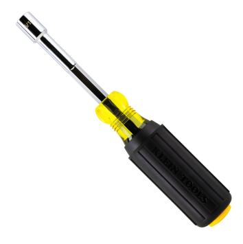
Klein's Color-Coded Hollow-Shaft Heavy-Duty Nut Driver features a fully pass through driver for driving nuts on threaded rod and prevents bottoming out. Cold forged steel wrench assist provides greater torque, especially helpful for breaking stubborn nuts and bolts free. The handle is color-coded and dome-stamped to easily identify the common 5/16-Inch hex size needed for the job.
