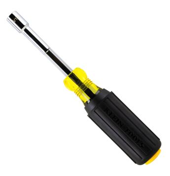
Klein's Magnetic Color-Coded Hollow-Shaft Heavy-Duty Nut Driver features a fully pass through through drivers for driving nuts on threaded rod and prevents bottoming out. Rare-Earth metal magnet is protected by a brass inner sleeve and strike plate to prevent the magnet from falling out or being damaged by sharp edge threaded rod. Cold forged steel wrench assist provides greater torque. Color-coded handle and dome-stamped to easily identify the common 5/16-Inch hex size needed for the job.
