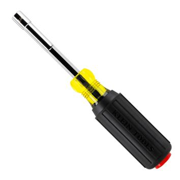
Klein's Magnetic Color-Coded Hollow-Shaft Heavy-Duty Nut Driver features fully pass through drivers for driving nuts on threaded rod and prevents bottoming out. Rare-Earth metal magnet is protected by a brass inner sleeve and strike plate to prevent the magnet from falling out or being damaged by sharp edge threaded rod. Cold forged steel wrench assist provides greater torque. Color-coded handle and dome-stamped to easily identify the common 1/4-Inch hex size needed for the job.
