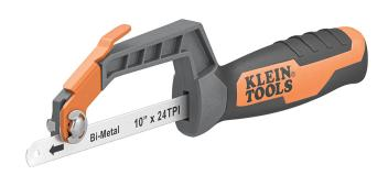
The Klein Tools Compact Medium-Cut Hacksaw is designed to cut most plastic, wood, and thin wall metal tubing. The saw has a 10-lnch by 24 TPI bimetal hacksaw blade that is easy to adjust and exchange by engaging the tool-free lever.
