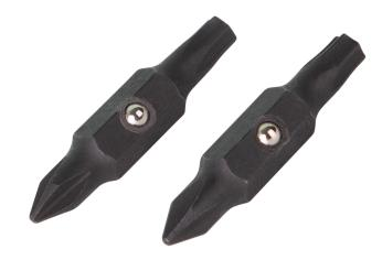
Replacement bit for Klein's Heavy-Duty and Ratcheting Multi-Bit Screwdriver/Nut Drivers. #2 Phillips and T25 Tamperproof TORX® tips are precision machined for exact fit into fastener. The heat-treated bits are industrial strengths for the ultimate in durability and performance.
