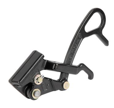
The Klein Tools Wide Range Service Grip is a versatile, one-handed grip designed to securely pull steel, ACSR, AAC, and Copper wires. Holds a wide range of common cable sizes from #6 to 4/0. This grip has a 2000-Pound maximum safe load.
