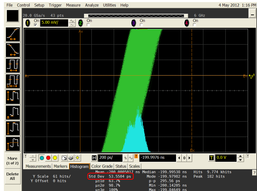
Figure 4. Jitter measurement on DDS signal
