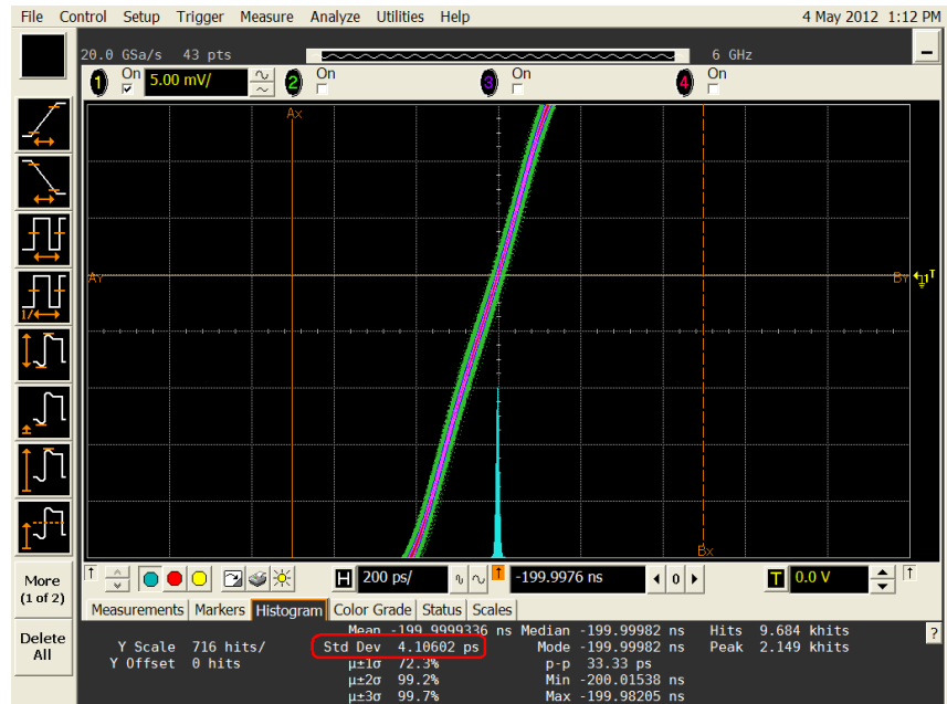
Figure 3. Jitter measurement on Trueform signal
