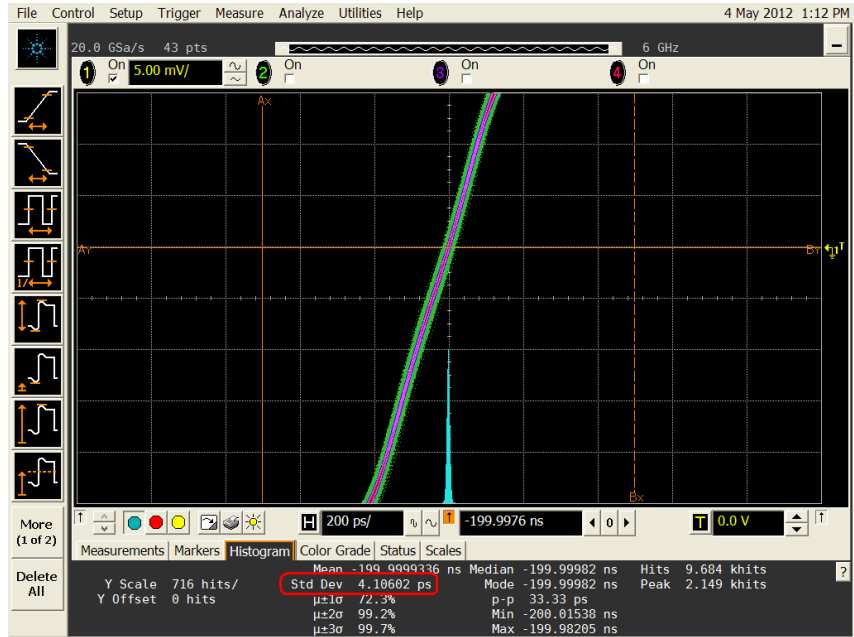
Figure 3. Jitter measurement on Trueform signal
