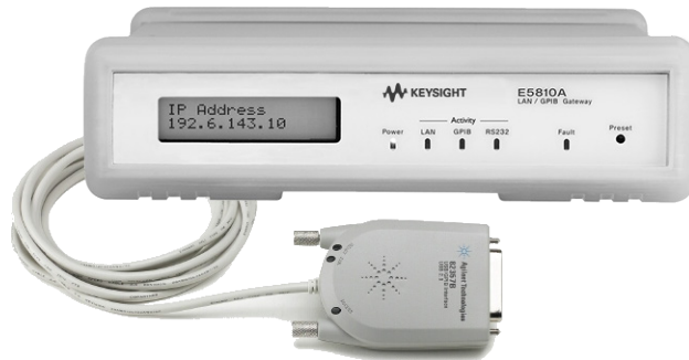
Figure 1. The Keysight 82357B USB/GPIB interface and E5810 LAN/GPIB gateway enables easy connection between PCs and GPIB instruments
