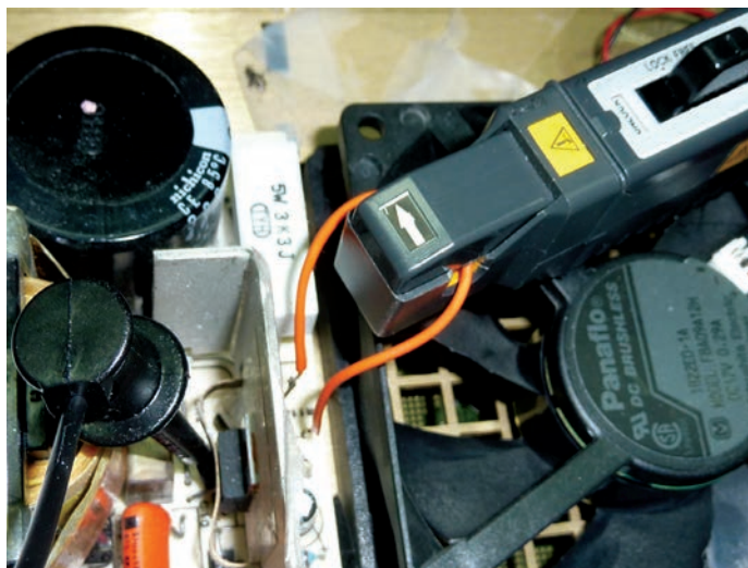
Figure 4. Creating a special current loop in your power supply to measure current.
