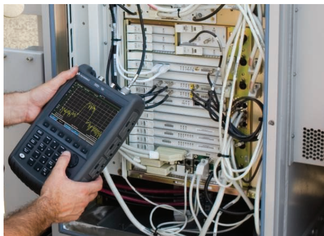
Figure 1b. FieldFox directly connected to a feeder line on a wireless communication system
