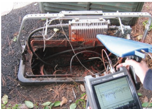
Figure 1a. FieldFox connected to a directional antenna for locating a source of radio interference
