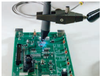
N2795A/96A comes with a headlight for better visibility while probing
