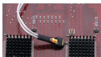
N5439A InfiniiMax III ZIF probe head soldered in to an IC
