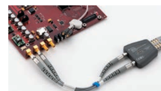
N5444A InfiniiMax III 2.92-mm SMA with N5448A SMA flex cable connected to a SMA connector on the board
