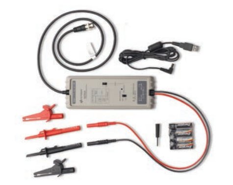
N2791A 25-MHz, 700-V differential probe with standard accessories
