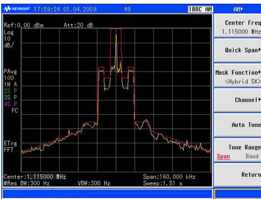
IBOC-AM measurement with N9340B IBC
