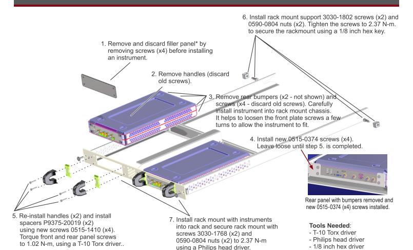
Installation of 1-High Rack Mount with Two Instruments \*Filler panel is only removed/discarded in a 2-unit installation.
