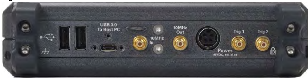
Figure 1-11 P937xA Rear Panel
