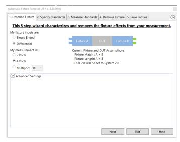
through characterizing a fixture and removing it from the measurement. Devices can be single-ended or differential. Files can be saved in a variety of formats for later use in Streamline Series VNA.
