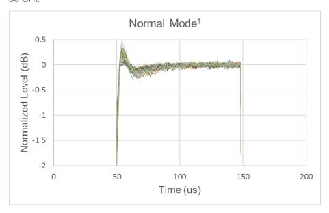
1. Measured with a 500 kHz IF bandwidth, averaging factor of 16 (Average Type = Point). With 100 us pulse width setting. 50 nsec/div.
