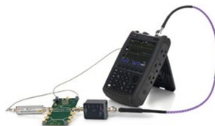
Accurately characterize noise figure of devices
