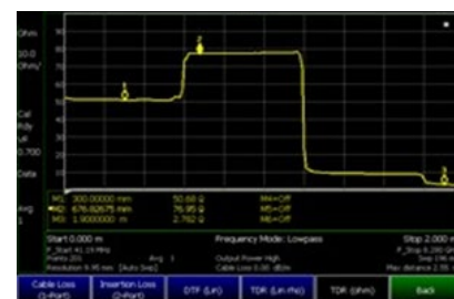
Gain insight into faults with TDR measurements
