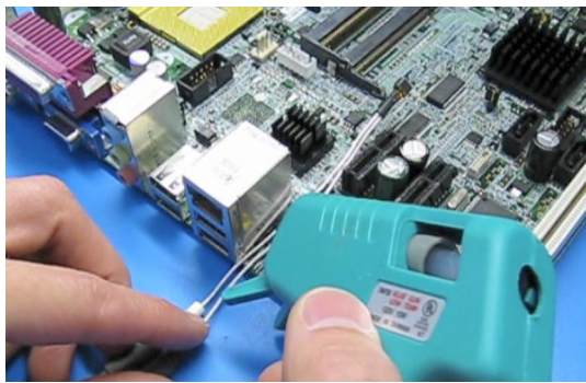
Figure 60 Probe Secured Using Low-Temperature Hot Glue
