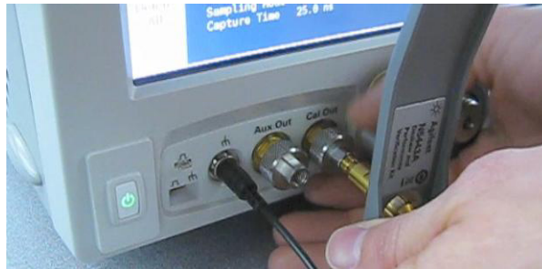
Figure 75 Attaching the N5443A Fixture
