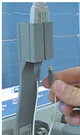
Figure 79 Connect the Head to the Probe
