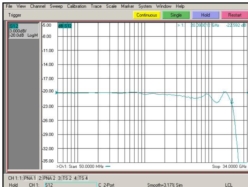
Figure 106 De-Embedded V_{out} Trace
