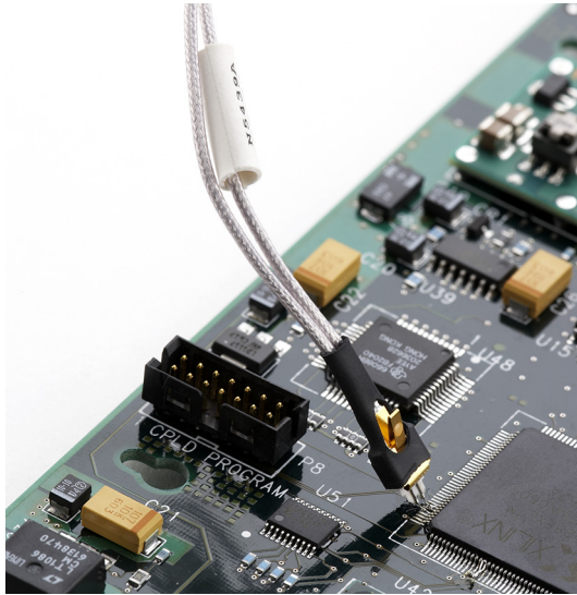
Figure 32 Probe Oriented Perpendicular to Device
