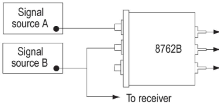
Figure 4. Multi-source switching
