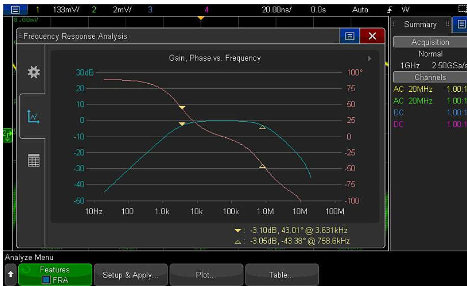
Figure 28. Frequency response analysis plot (Bode gain & phase) of a bandpass filter.
