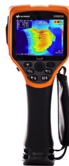
Figure 17b. Keysight U5855A TrueIR thermal imager
