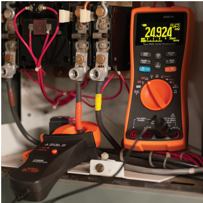
Figure 1. Measure current drawn on the hot wire with AC current clamp
