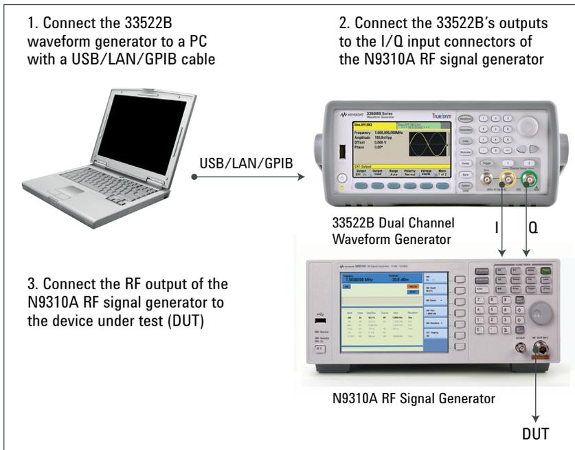
Figure 1. System setups for creating GFSK signals
