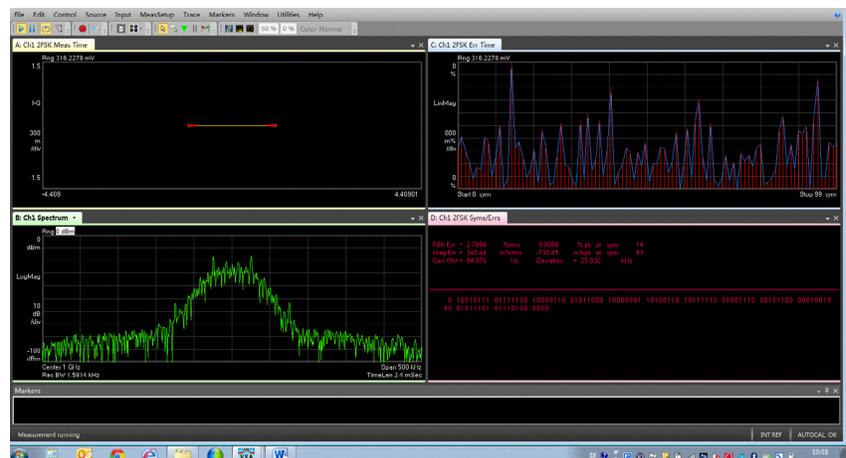
Figure 2. Verifying the GFSK signal with Keysight VSA software
