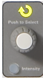
Figure 7 Oscilloscope general-entry control
