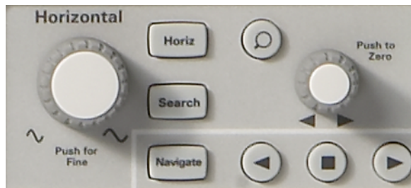
Figure 4 Oscilloscope horizontal (X-axis) controls
