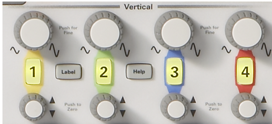
Figure 5 Oscilloscope vertical (Y-axis) controls
