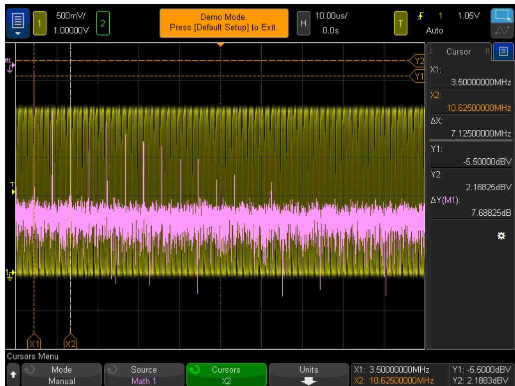
Figure 43 Performing an FFT math function on a repetitive digital clock
