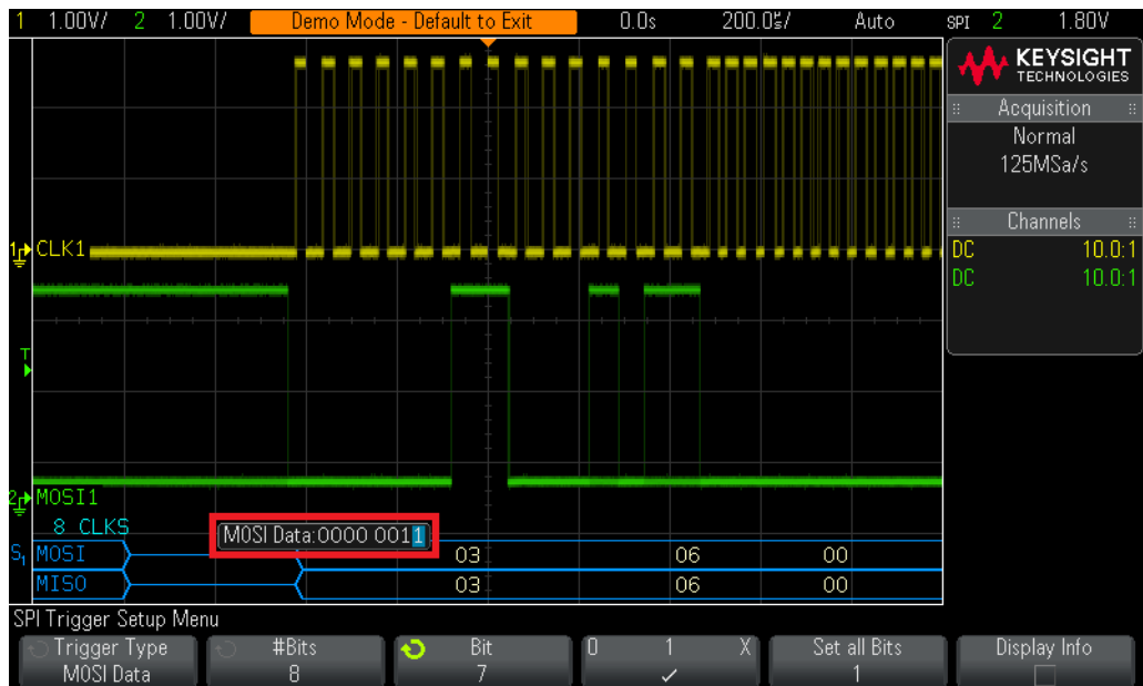
Figure 40 Triggering on MOSI data = 03 HEX .
