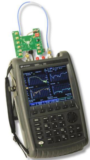
Figure 7. (a) Amplifier test bench using benchtop equipment and (b) the equivalent test setup using a handheld FieldFox combination analyzer
