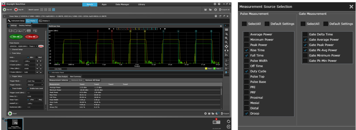
Figure 10. Multi-channel trace display with 4-pairs of gates and automatic pulse parameters measurement (sample screen shot with two U2042XAs).
